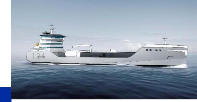
T-24 tanker will have an option for pre fitting oil recovery system.
