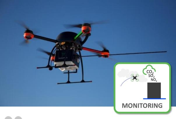
This project demonstrates the applicability of the ultra light Aeromon BH-8 sensor module and the real time reporting tool, Aeromon Cloud service in emission monitoring."
