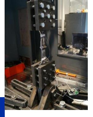
This Tekes funded project executed in cooperation with Lappeenranta University of Technology deepens the knowledge of the effect of corrosion to the endurance and strength of steels as well as the effect of low temperature to the strength and fatigue of differently manufactured steel products, especially welded structures.
